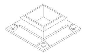
SPOT FACED FOR VERTICAL 7/16" DIA. HOLES FOR 3/8" DIA. ANCHORS
