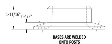
2-1/2" SQ. POST FITTED WITH 2.3" SQ. x 1/4" WALL x 3-5/8" LONG 6063-T6 REINFORCEMENT BAR
