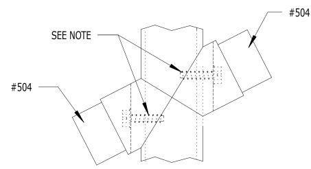
\*\*THRU BOLT (#524) AND LOCKNUT (#525)
