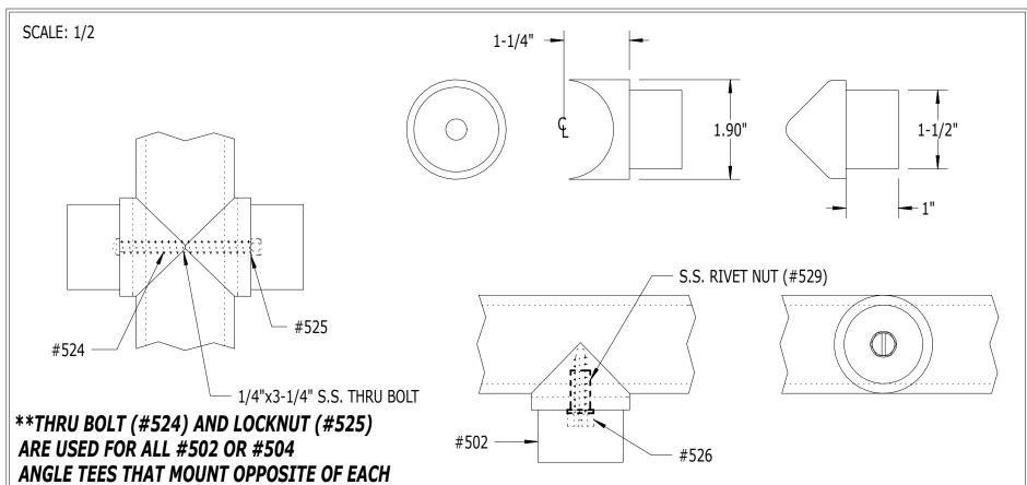
\*\*A STAINLESS STEEL RIVET NUT (#529) AND A  $1/4" \times 1-1/4"$  S.S. SCREW (#526) ARE USED ON ALL TEE OR ANGLE TEE LOCATIONS THAT ATTACH TO JUST THE PIPE, AT ANY DEGREE.
