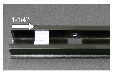
Next, use a hacksaw or a cut off saw and cut to the required length. Remove any burrs from the sawcut. Finally, reinstall the rail wedges 1-1/4" from the end of all the horizontal rails.
