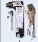
Each cable order comes with a 3/16" Allen Wrench with socket drive (A), a tension gauge (B) a cable gripping pliers (C)
